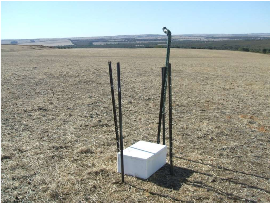
Plate 1: Bat Detector and Microphone Protector located at Sampling Point W3. Note Cattle Protection Rods
